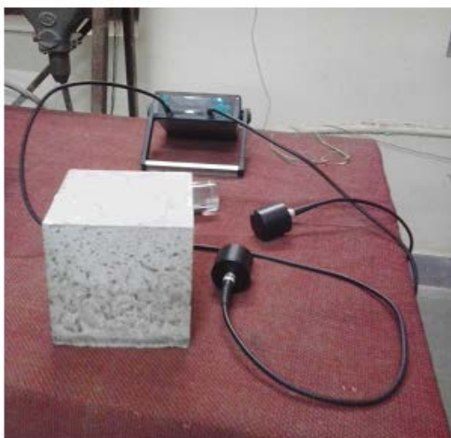
Fig 4. Performing ultrasonic pulse test for concrete samples.
