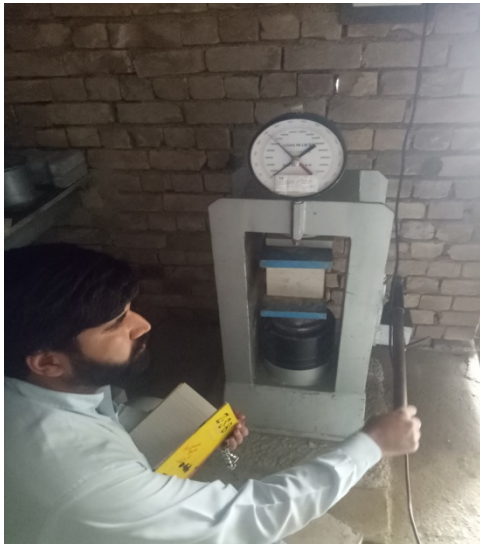
Fig 2. Performing of compressive strength tests using compression testing machine.
